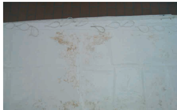
Example of moulding for wrongly stored temporary structures. It is clearly to see that mould has formed at the internal part of the folded material, probably due to the fact that the material was stored wet or that the storage place was not adequately dry.
