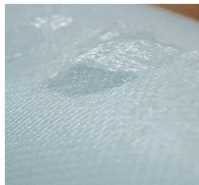
Image 1: "peeling effect" due to exaggerate lacquer thickness and bad adhesion.
