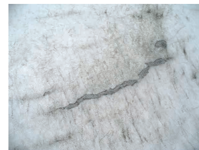
Image 3: Effect of stiffer surface due to thick lacquers. In some circumstances the lacquer substrate can generate deep cracks to the PVC coating.
