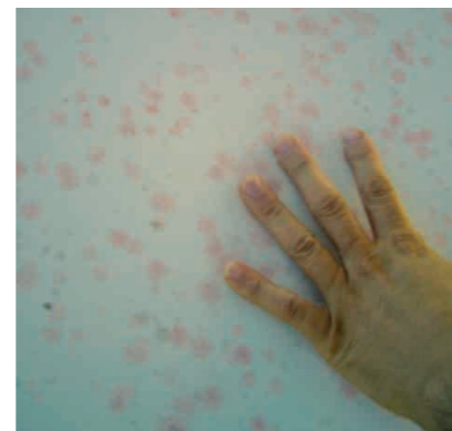
Fabric under fungal attack. Micro organisms have already invaded the coating with possible deteriorating of the original material characteristics.
